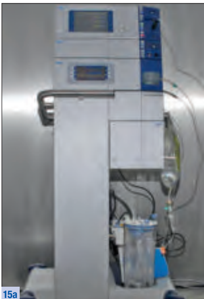
15a A water-jet scalpel (third generation Hydro-Jet dissector, Erbe, Tübingen, Germany) can be introduced through the integrated working channel of the new arthroscope (KARL STORZ GmbH & Co. KG, Tuttlingen; see Fig. 15c ).
